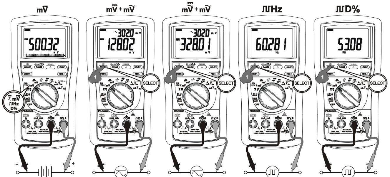
**ACmV +Hz, dBm +Hz, Hz +ACmV functions**
