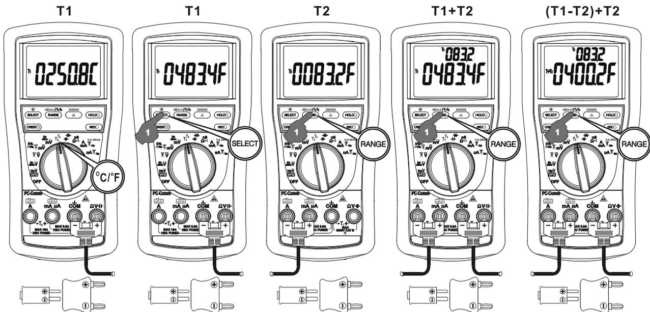
Note: Be sure to insert the banana plug type-K temperature bead probe AMD 9023 with correct **+** **-** polarities. You can also use a plug adapter AMD 9024 (Optional purchase) with banana pins to type-K socket to adapt other standard type-K mini plug temperature probes.
