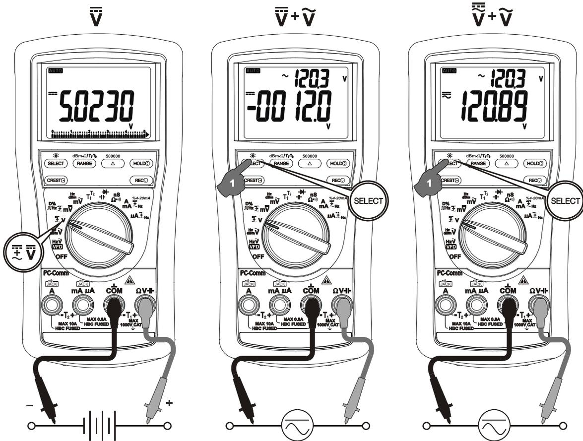
**DCmV, DCmV +ACmV, DC+ACmV +ACmV, Logic-Level  $\square\square$  Hz, Duty% functions**
